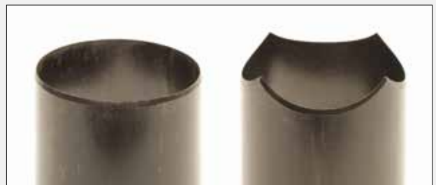
Outside sharpened: push up native soil
