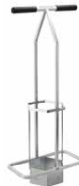
502108 7 in. (18 cm) Hex-Plugger, Cuts 3 in. (8 cm) Deep Plug
